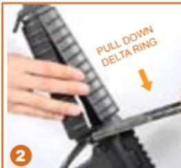
2. Use a handguard removal tool to pull down Delta Ring and remove the handguards.
