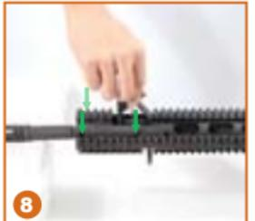
8. Tighten the four screws with the provided Allen wrench to lock the Bottom Extension with the Top Cover.
