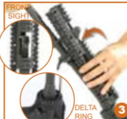
3. Install the Top Cover onto the barrel by aligning the inner two spinal cords against the central groove area on the barrel nut, and push for a tight fit. Make sure the Front Sight goes into the rectangular cut of the Top Cover.
