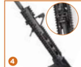
4. Press downward the Top Cover to pull back Delta Ring, and then release toward the barrel to allow the Front Cap to fit snugly inside the transversal channel in the middle of the Top Cover. Make sure that the Top Cover is evenly situated.
