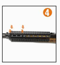
Tighten all 4 screws using the provided Allen wrench to secure the top and the bottom rail systems. The quad rail is now ready for most versatile accessory applications.
