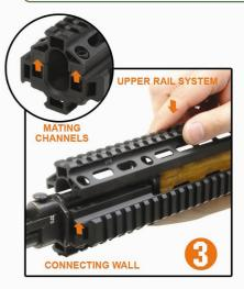
Fit the Upper Rail System onto the gas tube as shown. Make sure the 2 Connecting Walls of the Lower Rail System sit into the 2 Mating Channels of the Upper Rail System.
