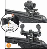
This claw mount comes pre-installed with a Picatinny rail ready for any Picatinny application. To use the mount for STANAG applications, remove the top rail by unscrewing the 2 Locking Screws from its underside using a flathead screwdriver. Re-use the Locking Screws to install a STANAG device, such as a scope, on the claw mount.
