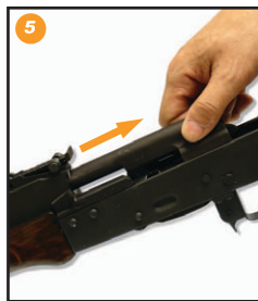
5. Remove the bolt and the bolt carrier, including the gas piston attached to the bolt carrier.
