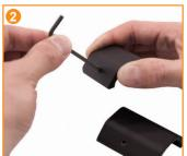
Using the included 3mm Hex wrench, install the two set screws in each of the barrel nut shims until the set screw heads are flush with the barrel nut shim's outer surface.
