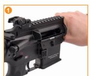
Make sure firearm is unloaded. Remove the HK handguard according to the instructions found in the HK user manual. Do not remove the HK gas block or barrel nut.
