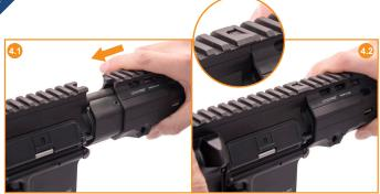
Hold the barrel nut shims in place and carefully slide the handguard on until the handguard's anti-rotation tab seats into the corresponding slot in the HK upper receiver flat top. Slight adjustments to the positioning of the shims may be required until proper alignment is achieved.
