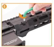
Using the included T30 Torx wrench, insert the handguard locking bolt through the right side of the handguard and turn clockwise to tighten. Recommended torque value is 40 in-lb.
