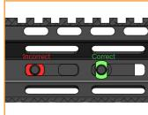
If the T-Nuts are spaced with too much gap they will rotate freely when trying to tighten. Alternately, if the T-Nuts are not spaced with enough gap they will not rotate at all. Observe the T-Nut during the installation process to be certain that they have rotated to their correct position as shown.
