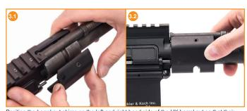
Position the barrel nut shims on the left and right hand side of the HK barrel nut so that their cutouts are facing down and are flush and in line with the channel found on the HK Barrel nut.
