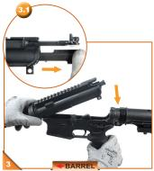
Remove the lower receiver with stock assembly. Take out the bolt assembly (3.1).
