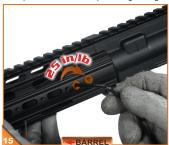
Once you achieve the proper alignment of the threaded holes on the Locking Ring to those on the handguard rail, use 6 of the Locking Screws to securely lock the handguard to the
