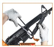
Remove the original plastic handguard with a handguard removal tool.
