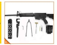
Prepare the rifle, the mount and necessary tools (an AR-15 combo wrench, 3mm Allen wrench, an AR-15 handguard removal tool, a hammer, a punch, an AR-15 upper receiver vise block, and a vise). Set up a comfortable working environment.
