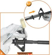
Securely place the barrel on a well padded flat surface. Punch the two pins at the bottom of the front sight out with a hammer and a punch. Remove the front sight with the gas tube, and take out the front cap (5.1)
