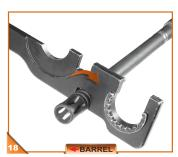
Install the flash hider on the Barrel.
