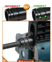
Make sure none of the 6 threaded screw holes on the Locking Ring are blocked by the Barrel Nut (13.1). If necessary, tighten the barrel nut a little further to allow access to the 6 screw holes. MAKE SURE NOT TO EXCEED 60 ft/lb OF TORQUE.
