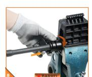
Fit the free floating Barrel Nut on the upper receiver and hand tighten. Test Alignment: Fit the handguard over the barrel and place over the Barrel Nut. Make sure the threaded holes on the hanguard align with the slots on the Barrel Nut (9.1-2). If the alignment is correct then move to step 10
