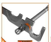
Remove the flash hider by turning it counterclockwise with an AR-15 combo wrench.
