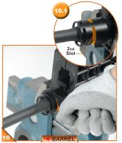
Place the Barrel Nut Wrench in the second slot (10.1) on the Barrel Nut (closer to the receiver) making sure the teeth of the Barrel Nut Wrench are fully seated into the 2nd slot
