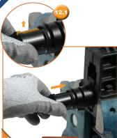
Slide the Locking Ring into the Barrel Nut, making sure the alignment slot on the Locking Ring (12.1) is vertical and facing upward.
