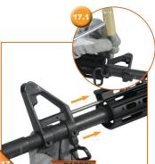
Reinstall the front sight to the gas tube. Reinstall the two pins to lock the front sight to the barrel (17.1).
