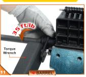
Using the Barrel Nut Wrench to securely tighten the Barrel Nut with enough tension (35 ft/lb). (We recommend using a torque wrench to achieve proper tension)
