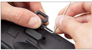
Place bolt catch detent over spring. Insert both as an assembly, spring-end first, into accompanying recess in the receiver. Insert bolt catch over assembly. While holding down the bolt catch down in place, insert the #6-32 pin so that the bolt catch is captured in place.
