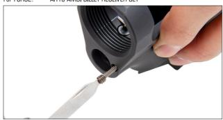
Insert takedown pin from the right side of the receiver with its channel facing towards the back of the receiver. Insert detent first and then spring into the accompanying hole in the back of the receiver. Ensure detent is captured within the channel.
