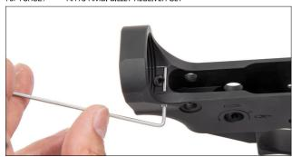
Place buffer detent over spring. Insert both as an assembly, spring-end first, into the accompanying recess in the receiver. While holding down the buffer detent in place, insert the steel retainer rod into the accompanying hole on the right side of the receiver and in through to the left side.
