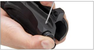
Place spring over forward assist. With the forward assist's claw facing inward towards the receiver, insert both as an assembly into the accompanying recess in the receiver. While holding down the assembly in place, insert the #6-32 pin so that the assembly is captured in place.
